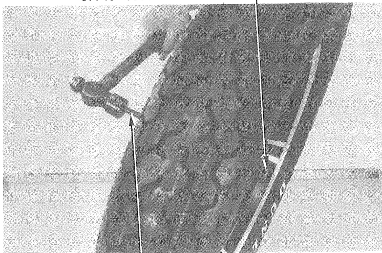
WHEEL BEARING REMOVER EXPANDER 07746-0050100 OR EQUIVALENT
