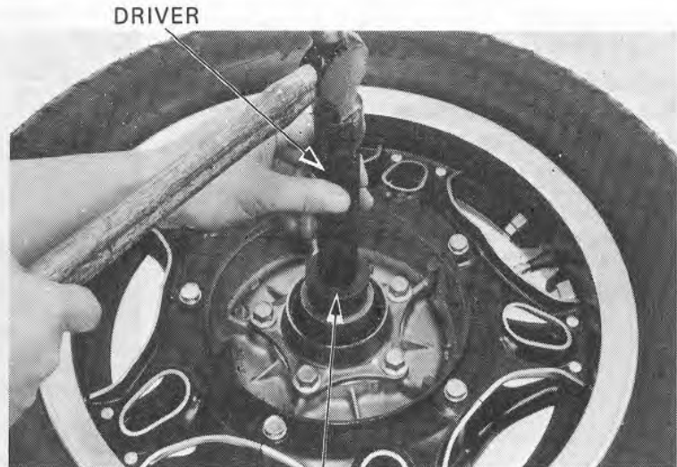
ATTACHMENT 42 x 47 mm AND PILOT 15 mm
