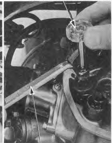
VALVE ADJUSTING WRENCH 10 x 12 mm
