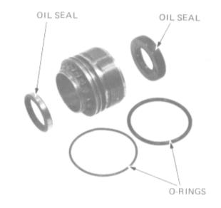
Fill the new oil seal groove with Multipurpose NLGI No. 2 (MoS<sub>2</sub> additive) Grease and install the oil seal into the retainer.
