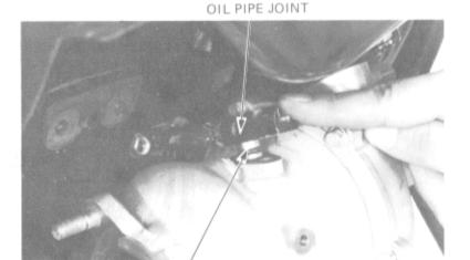
Install the exhaust manifold heat covers. Remove the tape from the oil outlet hole.
