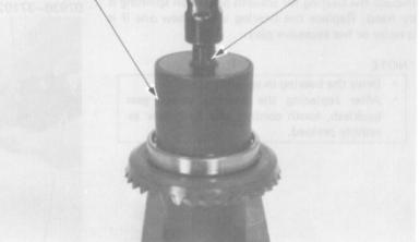
Install the ring gear bearing on the ring gear.
