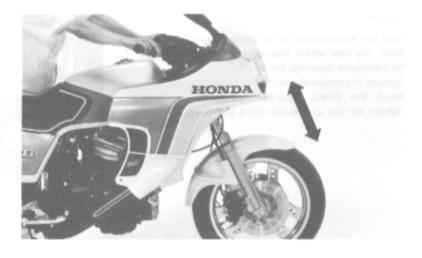
Check the front fork air pressure when the front forks are cold.
