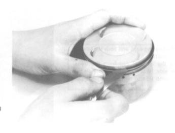
Insert each piston ring into the cylinder and measure the ring end gap.
