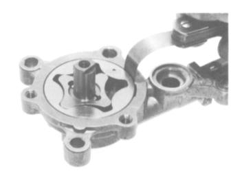
Measure the pump end clearance with a straight edge and feeler gauge.
