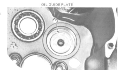
Install the mainshaft and countershaft bearings into the case.
