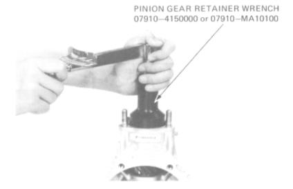
If preload is excessive, remove the preload inspection tool, then install the pinion gear retainer wrench and remove the retainer.
