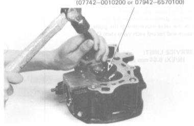
Place the Attachment on the Valve Guide Remover. Drive the guides into place from the top of the head.
